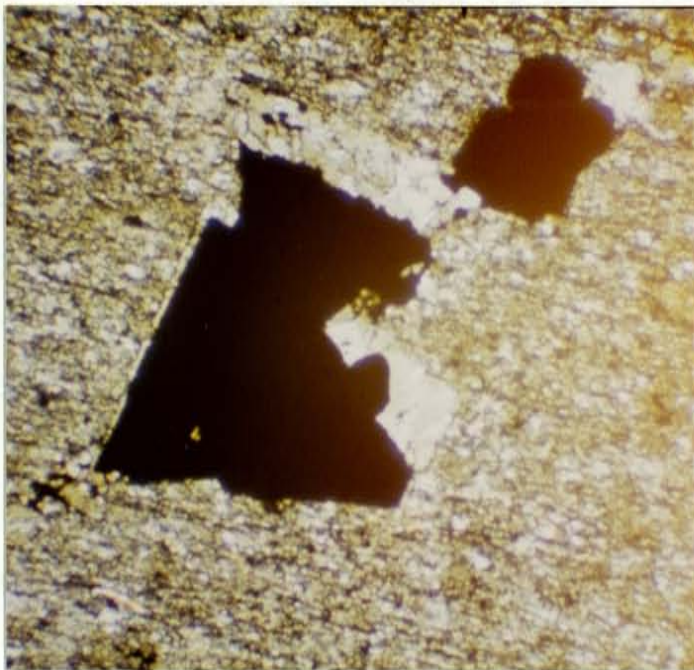
Figure 6a: Subhedral arsenopyrite (0.8mm) in fracture (0.2mm) in slate, crossed polars; sample 3027; scale: 25mm=0.5mm.
