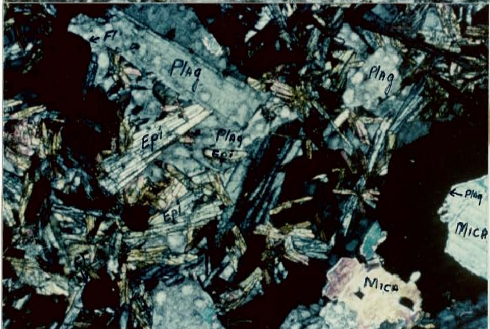
Figure 3. Ladron pluton, LD 80 epidote, fluorite and plagioclase crossed polarizers 40x
