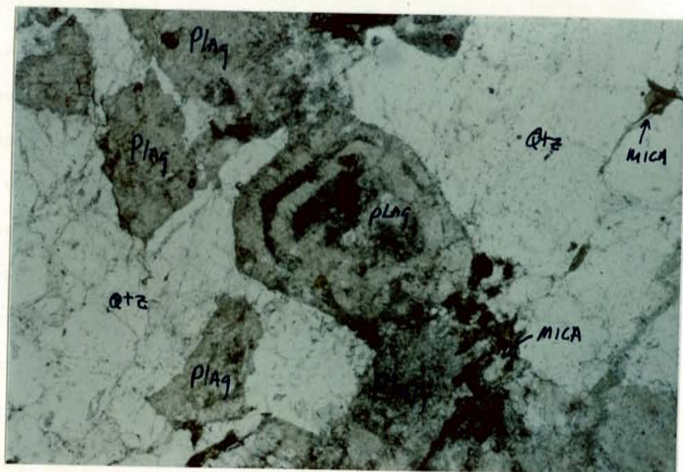
Figure 2. Ladron pluton, LD 7 oscillatory zoned plagioclase uncrossed polarizers 40x
