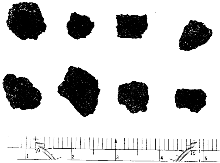
Figure 7: Fracture-bound clasts from Santo Tomas Mountain and Blackbird Hill showing generally equant form and fracture-bound surfaces.
