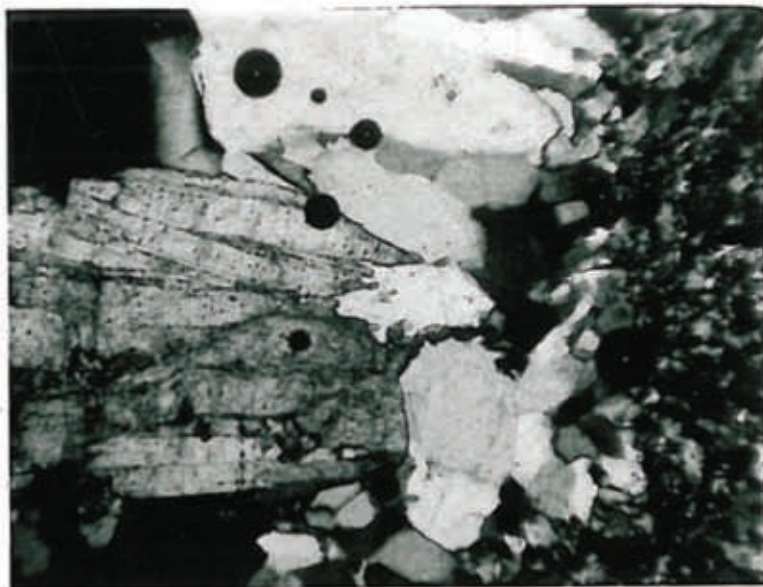
Figure 29. Barite growing in center of vein on crystalline quartz, which in turn is growing on microcrystalline quartz. Field of view is 2.0 x 1.45 mm. (crossed nicols).
