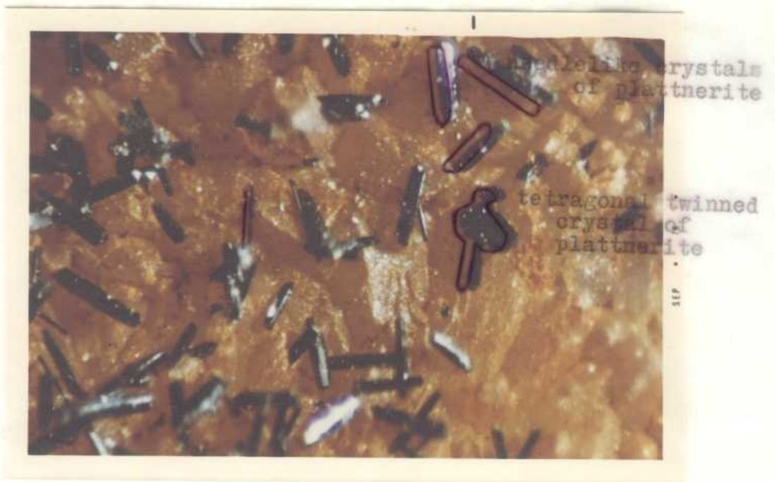
Photomicrograph showing shiny black needlelike crystals of plattnerite on goethite staining quartz. Tetragonal twinned crystals of plattnerite are also shown in the picture. (picture taken by J. Taggart)
