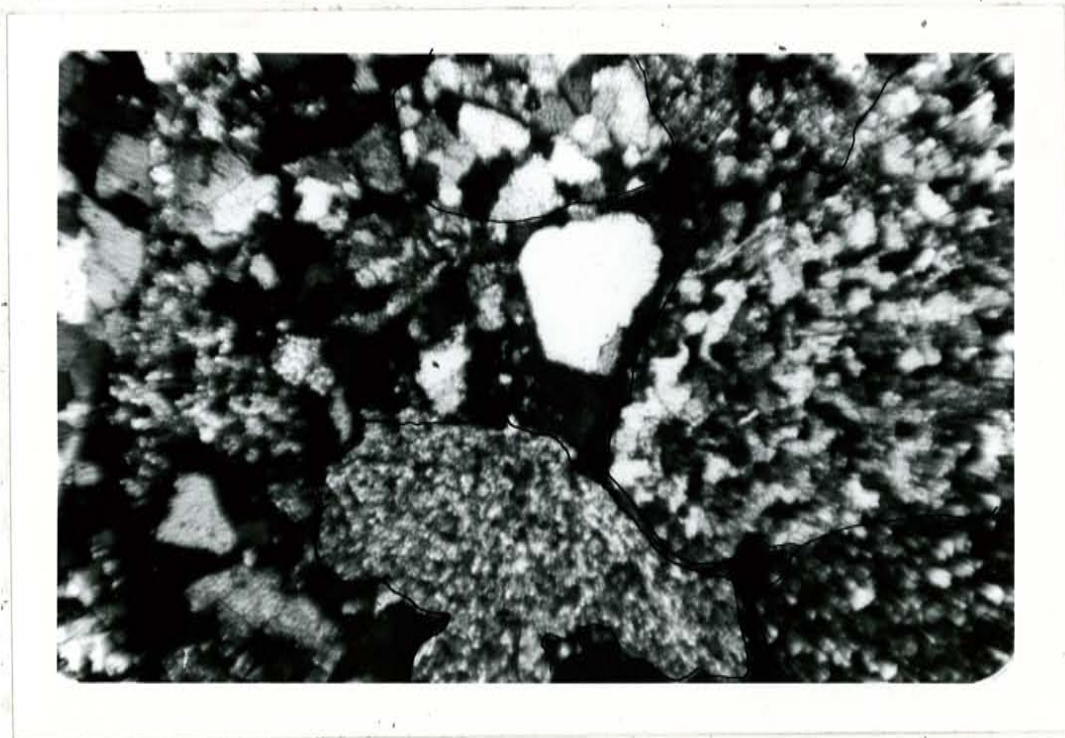
Figure 17. Photomicrograph of a typical T 1 Southern Sequence sandstone, X35, crossed nicols. Note the four quartzite rock fragments outlined in black and how the quartz in the fragments varies from very fine grained to coarse grained. Opaque iron oxide is common in these rock fragments. Note the absence of phyllite rock fragments and the abundance of hematite plus clay minerals matrix and resulting immature texture.
