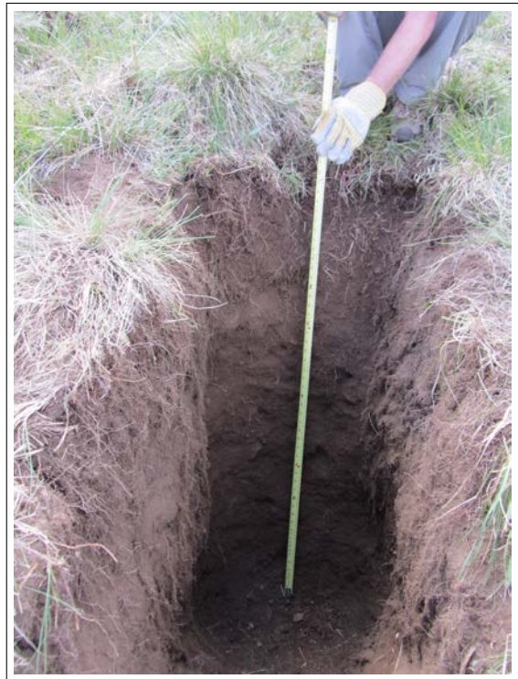
Figure 2.7: Soil pit dug into hillslope at about 3,577 m (11,735 ft) with tape measure for scale. Total depth was 1.4 m (4.6 ft) and bedrock was not encountered.
