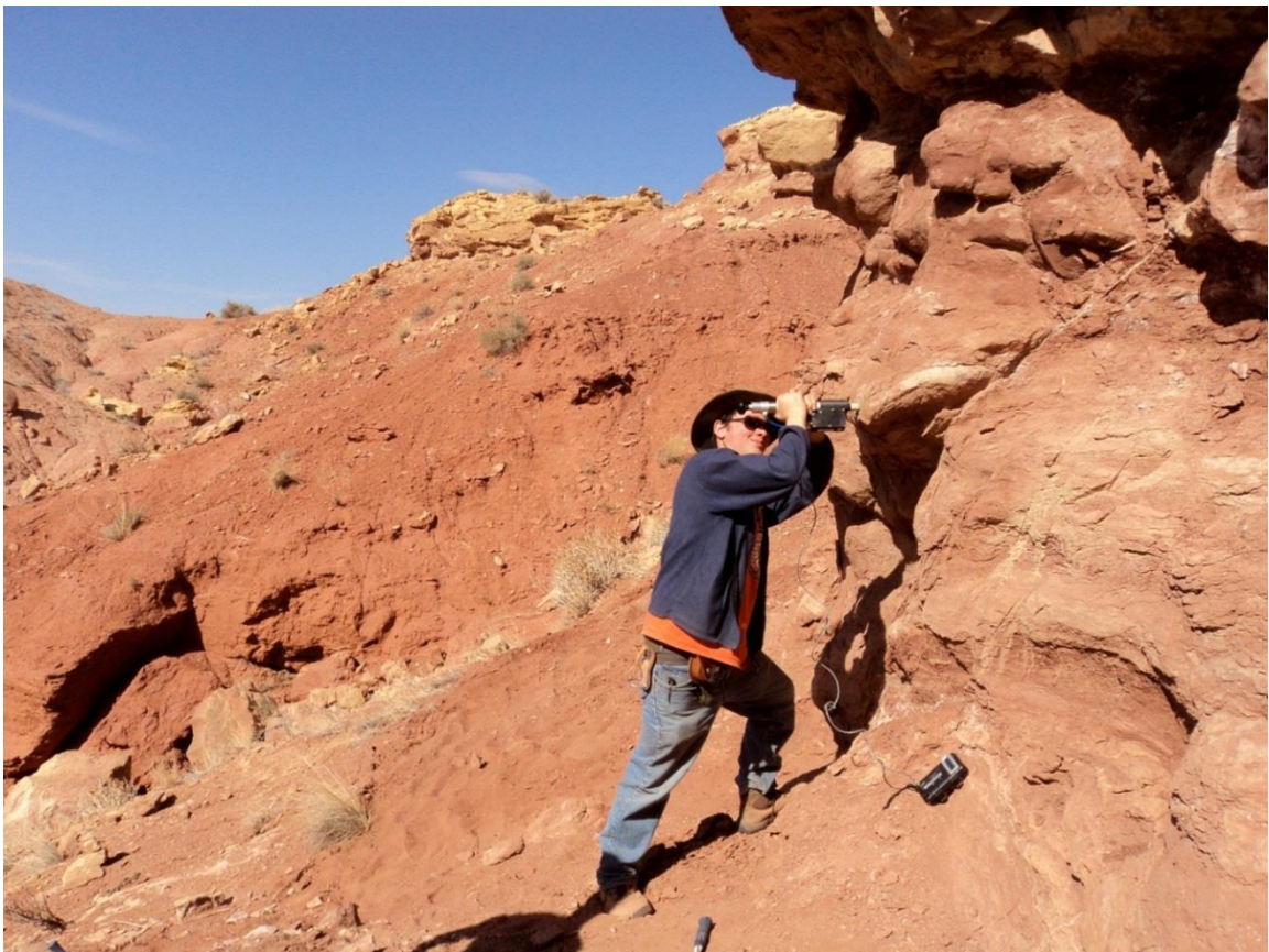
Figure 10. Using the TinyPerm II to gather permeability measurements in the field.
