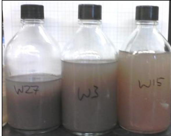
Figure 13. An example of turbidity observed in samples from the Sept. 23, 2011 sampling event. Samples displayed, from left to right, are from wells 27, 3, and 15.
