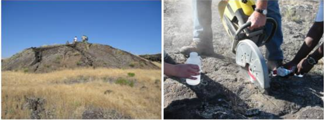
Figure 4.6: (left) Photo showing the type of landform (top of tumulus) sampled by the CRONUS project. (right) The Tabernacle Hill samples were collected using a saw and chisel.
