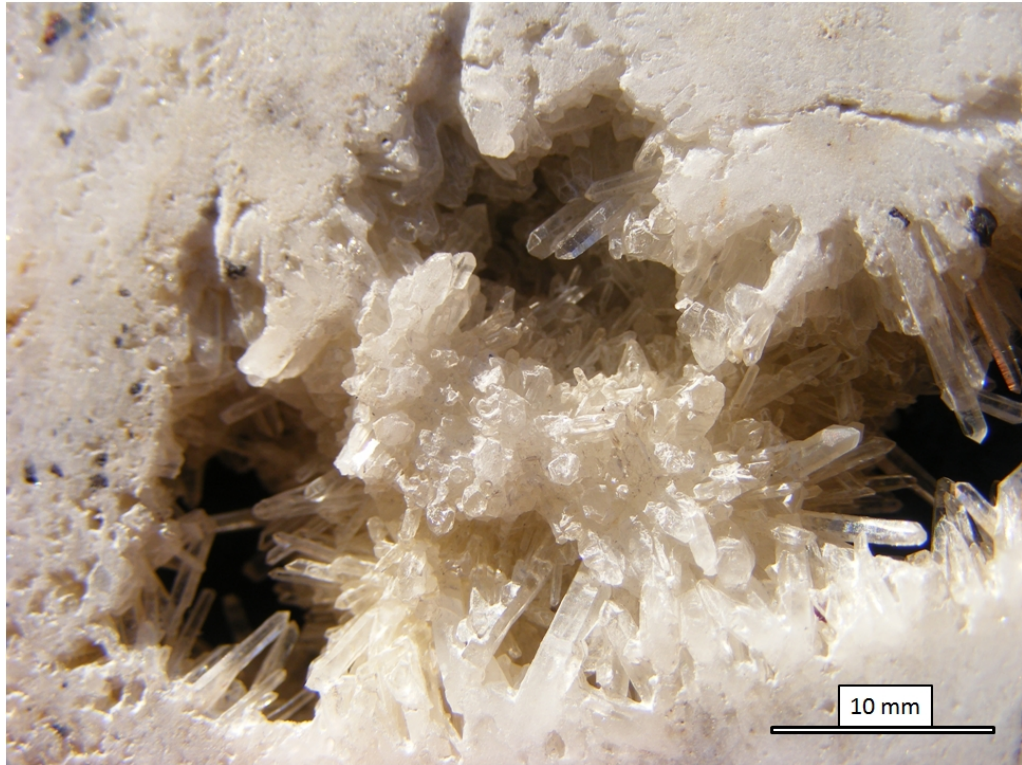
Figure 7.4: Copper Canyon sample showing a void in sample CCMM07 filled with well-defined quartz crystals. Crystal lengths range from 3-10mm.
