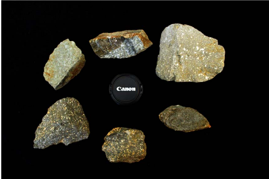
Figure 7. Tertiary andesite rocks from the alteration scars. Notice the dark green to brown color, which is remnant of propylitic alteration.
