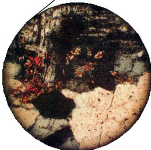
Photo micrograph of the contact between the groundmass and the qtz+cp vein. cp is found in the center of the vein. There is no altn halo associated with this vein.
