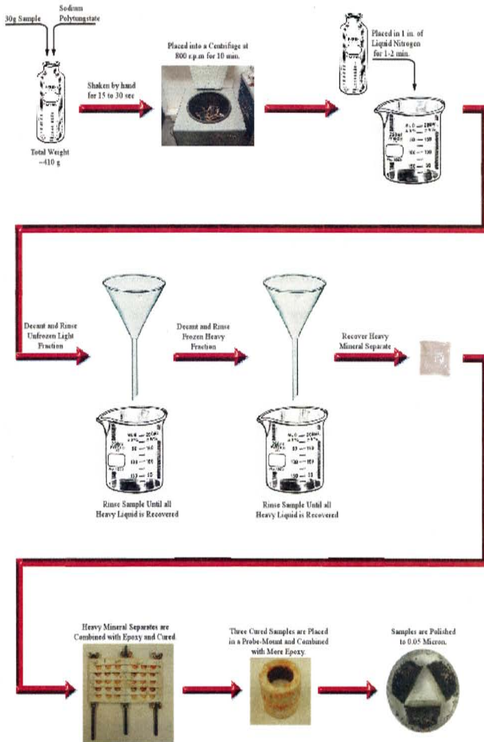
Figure 5.2: Sample preparation schematic for the heavy mineral separations. Each sample followed this separation procedure as illustrated above.
