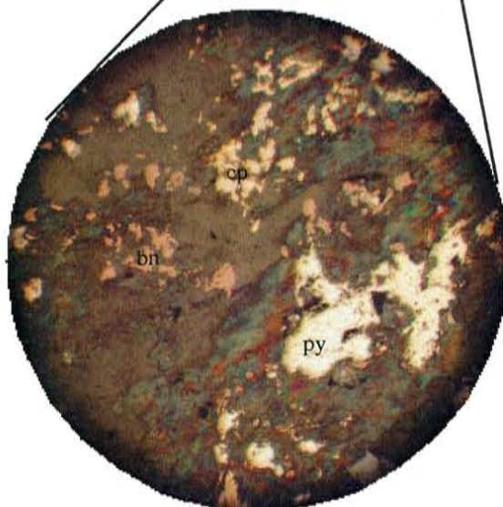
Photo micrograph of py+cp+bn mineralization associated with the development of qtz+ser+chl veins. There is no enrichment on hypogene sulfides.
