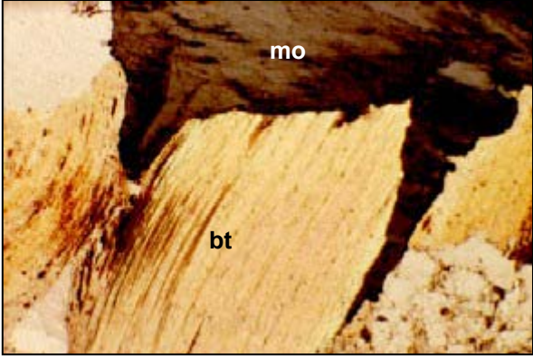
Mo filling bt grn boundaries in qtz-bt-mo matrix; trans and reflect; pln; 5x.
