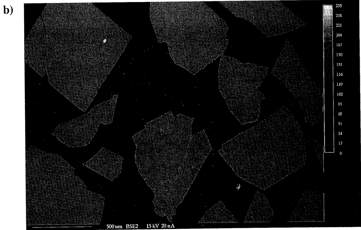
Figure 28 a-f. Representative back-scattered electron images of sanidine from each rock unit analyzed by electron microprobe. a) Vicks Peak Tuff (S085). b) Rhyolite lava (S069). c) Granite porphyry (S047). d) Rhyolite intrusion (S068). e) Rhyolite ignimbrite (S075). f) Turkey Springs Tuff (S071).
