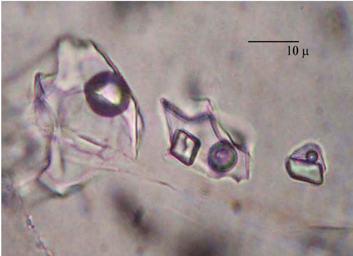
Figure 26. Photomicrograph of a group of secondary fluid inclusions that contain an unidentified solid + liquid + vapor (type III) in a fluorite crystal from sub-stage 3 of the mineralization stages. The photo shows a range of ratios between solid to liquid for each inclusion.
