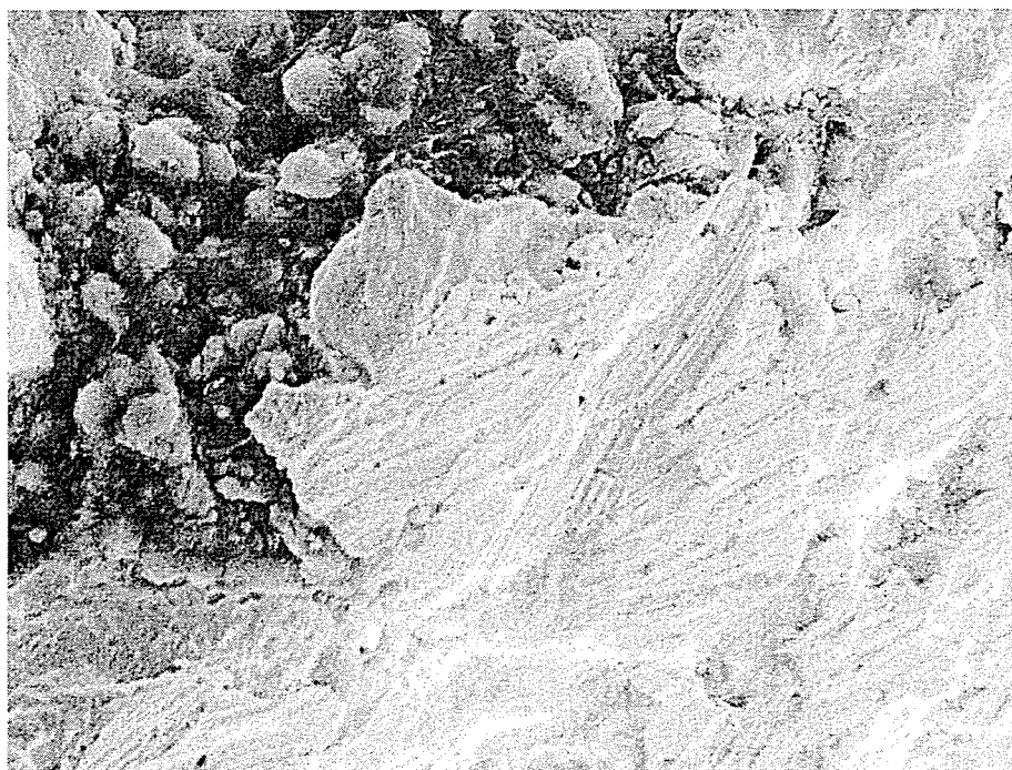
Figure 4.7 Electron microprobe image in SEM mode of a gold grain showing a close association with Fe-oxides (granular material). The field of view is about 100 \mu\text{m} .
