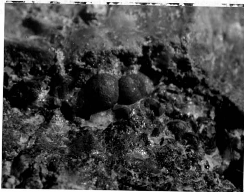
Figure 8. Typical lode tin occurrences in the Taylor Creek District. a) Nearly pure cassiterite (dark crystals) at the Squaw creek tin occurrence. b) Wood tin in chalcedony veinlet at the base of the carapace breccia in the Nugget Gulch tin occurrence. Large botryoids in center of photograph are about 2 mm diameter.
