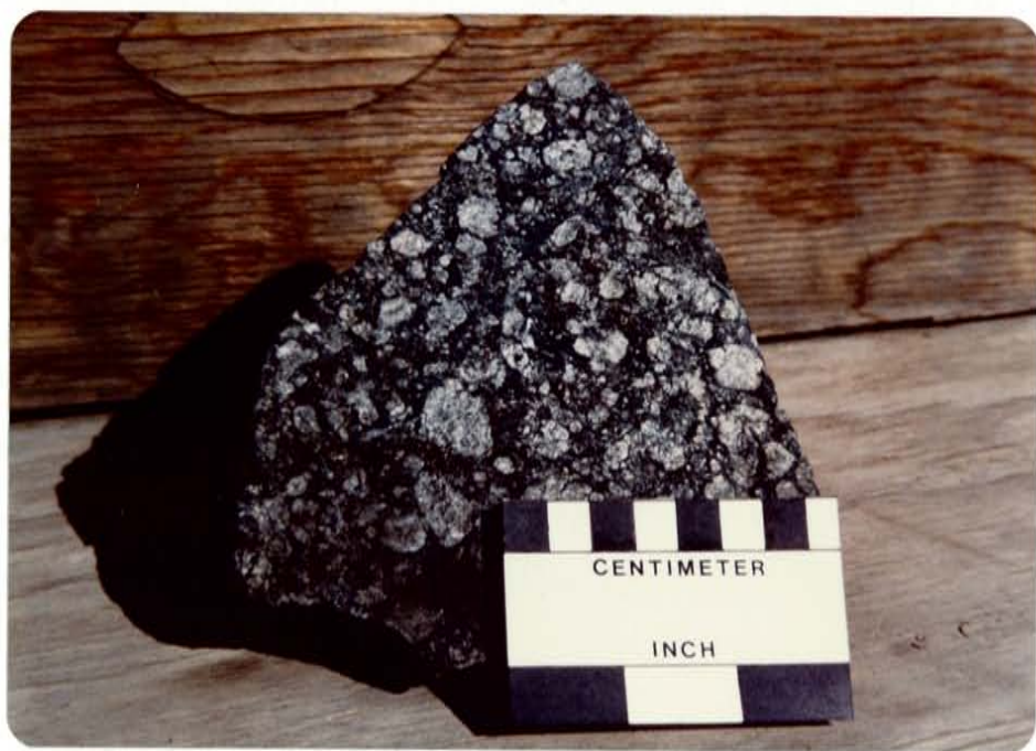
Figure 12. Cumulate plagioclase in porphyritic-amphibolite.
