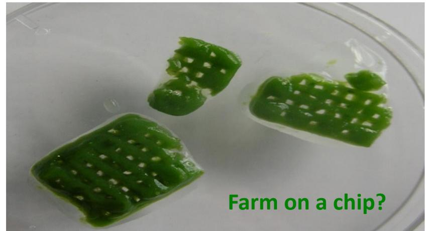
3D printed photosynthetic algae embedded in gel
