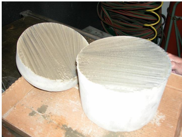
Figure 8 Cut specimen of cemented surrogate nitrate salt/Swheat
