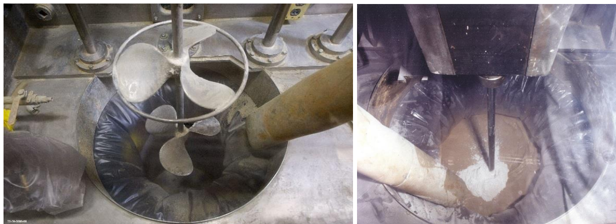
Figure 5 Cementation glovebox operation at TA-55
