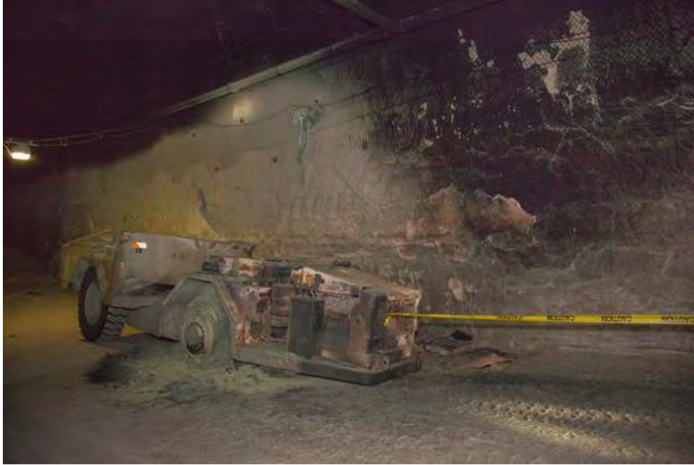
Figure 22: Haul Truck and Rib Spalling
