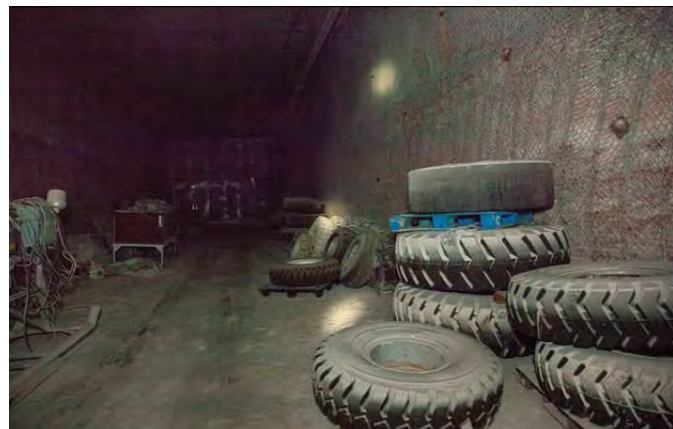
Figure 17: Combustible Loading in the Mine
