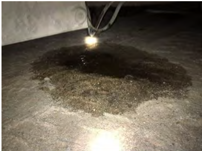
Figure 14: Hydraulic Fluid under Truck 74U006A
