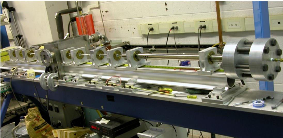
Figure 12: The SHPB apparatus at LANL (Courtesy of C. M. Cady)
