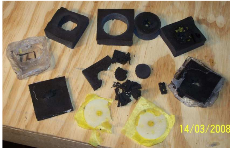
Figure 112: Damaged Foam Samples and Wave Shapers
