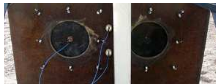
Figure 38: Separated Accelerometer Flat 35 ft Test
