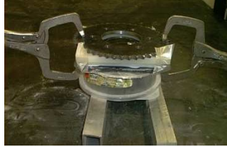
Figure 30: Setup to Manufacture a Dome Shape in the Foam
