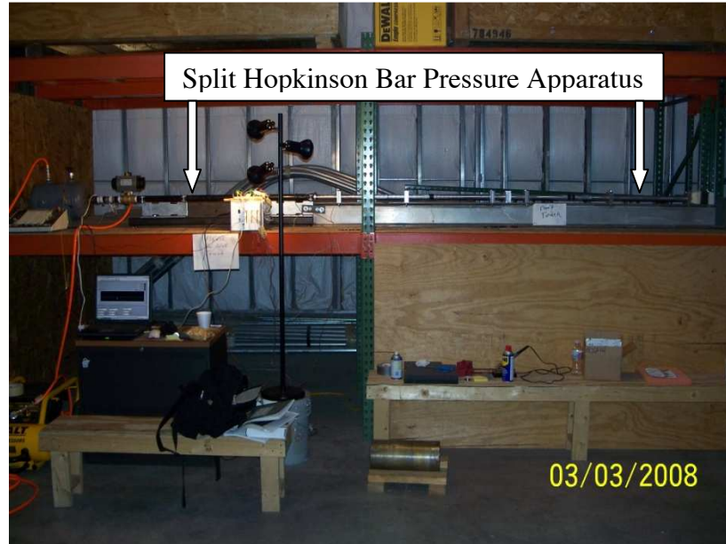
Figure 42: Split Hopkinson Bar in Built Room Iris Passcal Warehouse
