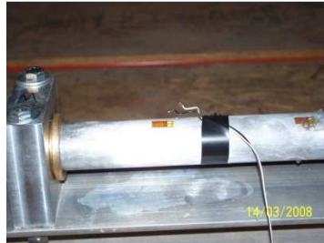
Figure 50: Vishay ¼ in 120 Uniaxial Strain Gage (Broken Solder Connections)
