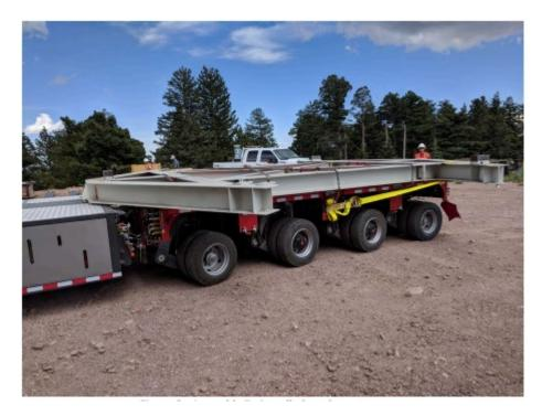
Figure 2: Assembly jig installed on the transporter.
