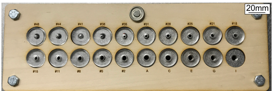
Figure 3.6: Circular orifice plates made for validation of opening area measurements placed in a laser cut wood organizer.
