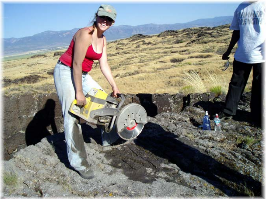
NMT graduate student Shasta Marrero wields a rock saw while sampling a late Pleistocene basalt flow at Tabernacle Hill, Utah, for the CRONUS-Earth Project.
