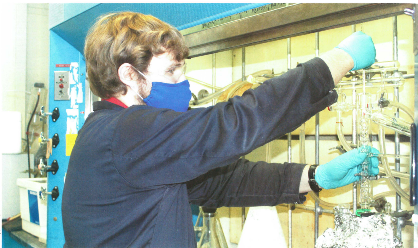
Chris Walking, a chemical engineer working in the NAWCWD research department, conducts a distillation of a biosynthetic fuel component.
